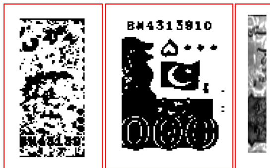
Figure 3: Left-most shows the extraction of the picture watermark, the central one shows the extraction of the serial number, and the right-most shows the security thread extraction of genuine note
