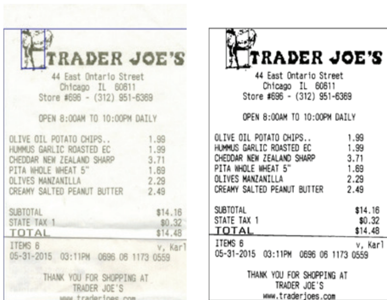
Figure 2: Trader's joe receipt before and after image binarization
