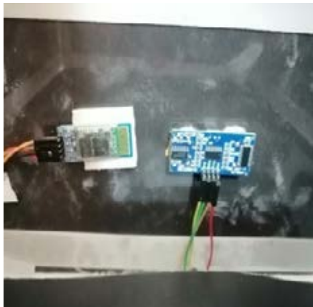
Figure 18: Integration of Arduino with Bluetooth module and Ultrasonic Sensor
