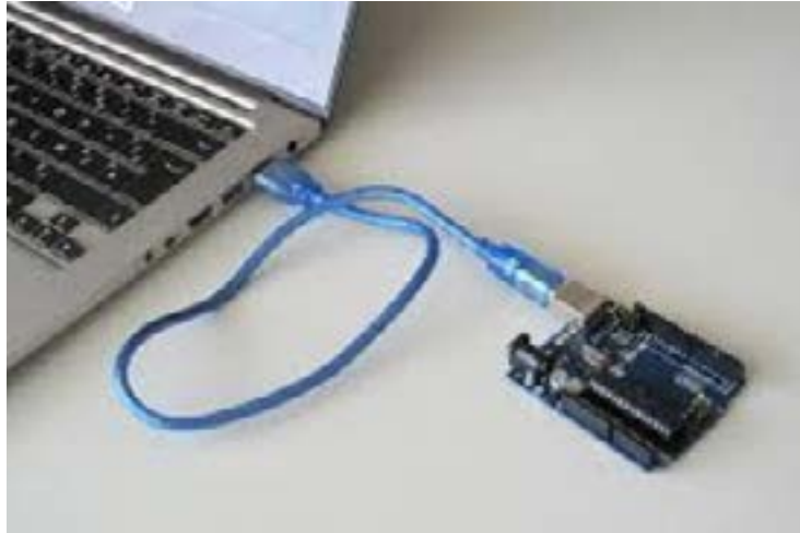
Figure 4. Arduino R3 interfacing with Computer
