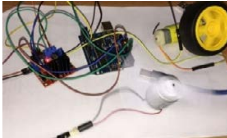
Figure 13: Motor Movement Based Testing Results of Arduino and L298N Motor Driver Module
